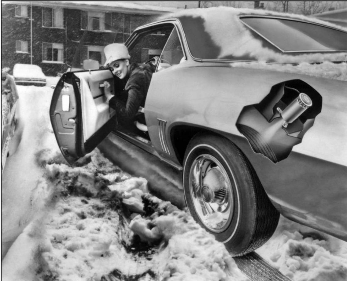
**The Liquid Tire Chain** Just over 2,600 Liquid Tire Chain systems made it onto the road across the 1969 Chevrolet lineup, with the vast majority installed on full-size Chevrolets. For reasons unknown, the V75 Liquid Tire Chain lasted for only a single year.
