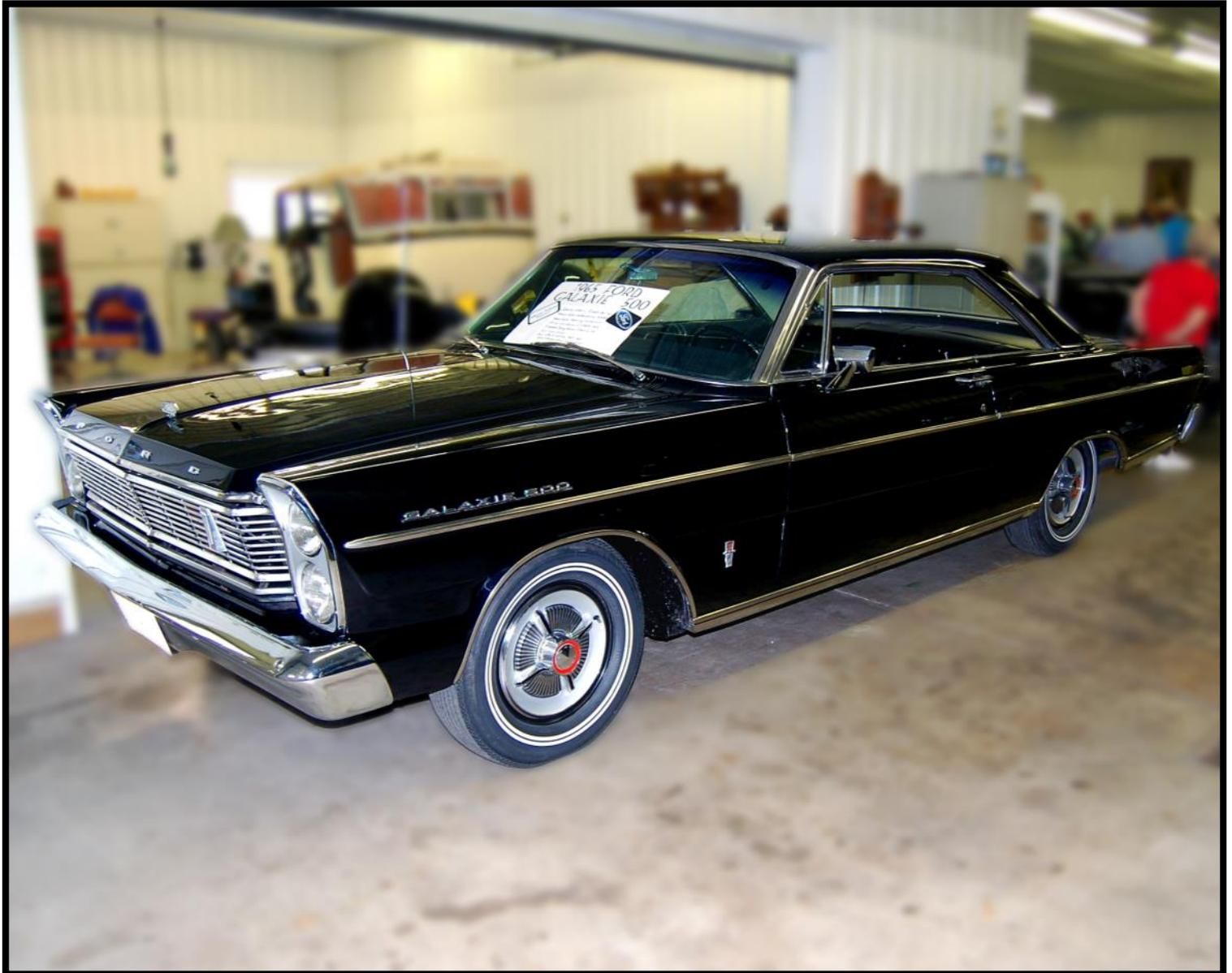
Wayne Scherer's 1965 Ford Galaxie 500. Special order— 8 week delivery. Heavy Duty riveted police brakes. Heavy Duty handling Police suspension. 390 cu. Inch engine w/ 4 barrel carb. 3 speed Borg Warner trans. w/OD. 300 horse power. Only 6% of entire 1965 had this transmission combination.
