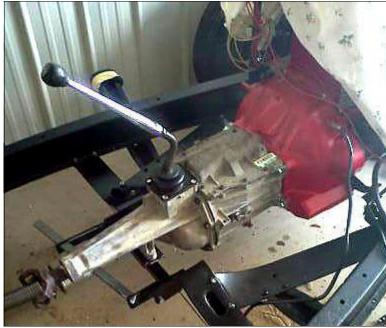
I recently obtained a T5 (transmission number 1352-145) with a 14 spline input shaft. The 1352-145 T5 gear ratios are 1st 3.76 2nd 2.18 3rd 1.42 4th 1.00 5th .072. They are out of an 1985 / 1986 L4 or V6 Chevy S10 PU. Transmissions of this vintage used mechanical speedometer. Later models may use an electronic sensor.
